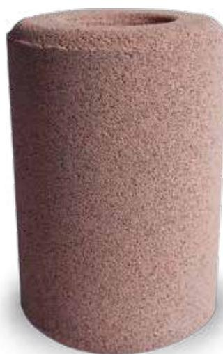
Elgin Cores with Replaceable Core Shell protect refrigeration and air conditioning systems against residual moisture, acids and solids. In addition, they are suitable for cleaning such systems. They can be used in new systems or in those whose compressor has been burnt. The sieve cores have low pressure drop and high drying capacity. Indicated for systems with HFC refrigerant fluids with Polyol Ester oil, HCFC and CFC Alkylbenzene and Mineral oil.
